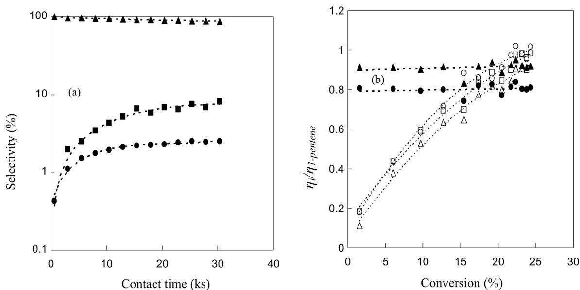
Fig. 2. (a) Selectivities of (▲) pentenes, (◆) cracking products and (■) oligomerization products during *n*-pentane dehydrogenation on Pt/Na-[Fe]ZSM-5 at 673 K in RRU unit in the absence of H<sub>2</sub>. (b) Ratio of ( $\eta_i/\eta_{1\text{-pentene}}$ ) as a function of *n*-pentane conversion: (▲) *trans*-2-pentene, (●) *cis*-2-pentene, (○) 3-methyl-1-butene, (△) 2-methyl-1-butene and (□) 2-methyl-2-butene. *n*-Pentane partial pressure: 25 kPa.
