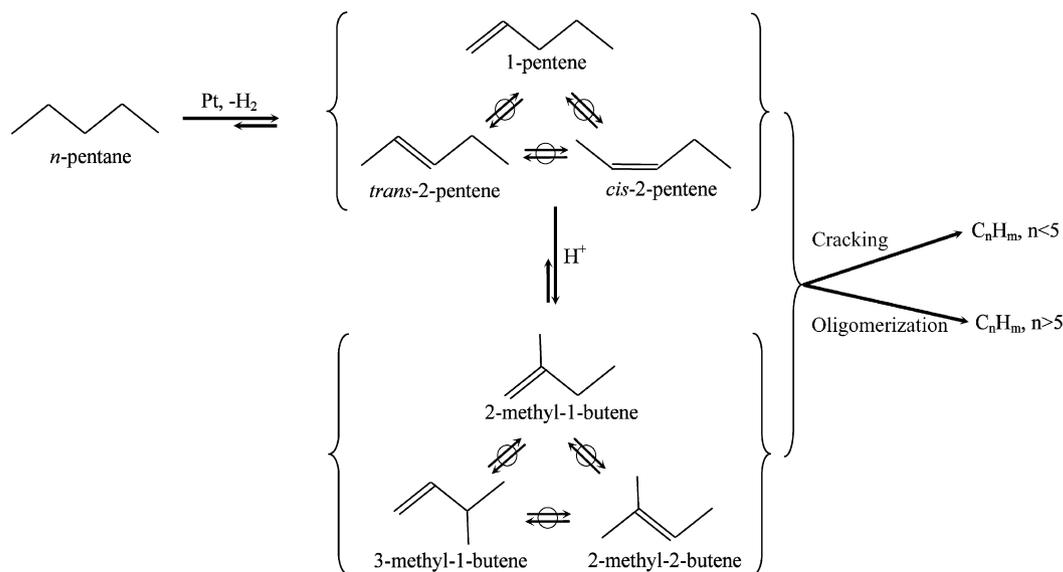
Scheme 1. Possible pathways for *n*-pentane dehydroisomerization on Pt/Na-[Fe]ZSM-5.
