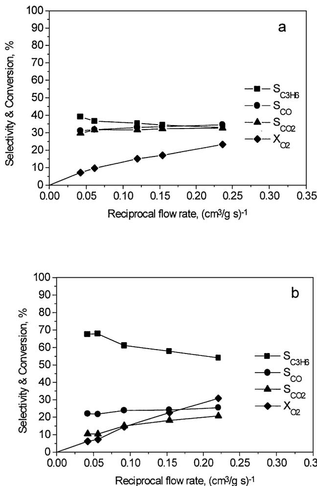
FIG. 7. Product selectivities and oxygen conversion for propane ODH over  $2\text{VO}_x/\text{ZrO}_2$  catalysts treated at (a) 673 and (b) 873 K. Reaction conditions:  $T = 606$  K;  $P_{\text{C}_3\text{H}_8} = 14.03$  kPa;  $P_{\text{O}_2} = 1.74$  kPa; weight of catalyst = 0.225 g.
