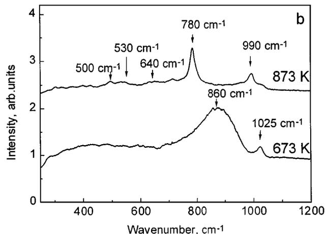
FIG. 4. Raman spectra of  $2\text{VO}_x/\text{ZrO}_2$  (a) and  $10\text{VO}_x/\text{ZrO}_2$  (b) samples calcined at 673 and 873 K.
