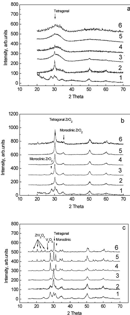
FIG. 2. XRD patterns of VO<sub>x</sub>/ZrO<sub>2</sub> catalysts calcined at 673 K (a), 773 K (b), 873 K (c) (1, ZrO<sub>2</sub>; 2, 2VO<sub>x</sub>/ZrO<sub>2</sub>; 3, 5VO<sub>x</sub>/ZrO<sub>2</sub>; 4, 10VO<sub>x</sub>/ZrO<sub>2</sub>; 5, 15VO<sub>x</sub>/ZrO<sub>2</sub>; 6, 30VO<sub>x</sub>/ZrO<sub>2</sub>).
