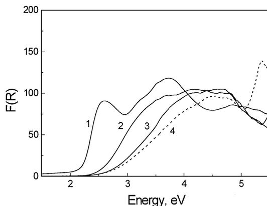
FIG. 5. Diffuse reflectance UV-Vis spectra of  $\text{VO}_x/\text{ZrO}_2$  catalysts calcined at 673 K (1,  $\text{V}_2\text{O}_5$ ; 2,  $30\text{VO}_x/\text{ZrO}_2$ ; 3,  $15\text{VO}_x/\text{ZrO}_2$ ; 4,  $2\text{VO}_x/\text{ZrO}_2$ ) and then exposed to ambient conditions.
