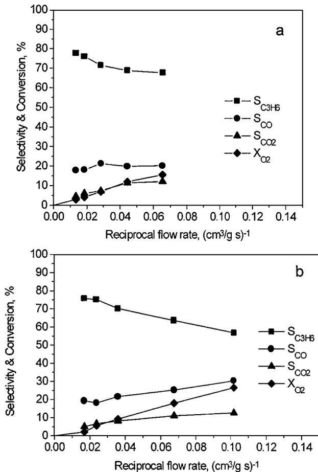
FIG. 8. Product selectivities and oxygen conversion for propane ODH over  $10\text{VO}_x/\text{ZrO}_2$  catalysts treated at (a) 673 and (b) 873 K. Reaction conditions:  $T = 606$  K,  $P_{\text{C}_3\text{H}_8} = 14.03$  kPa,  $P_{\text{O}_2} = 1.74$  kPa, weight of catalyst = 0.045 g.
