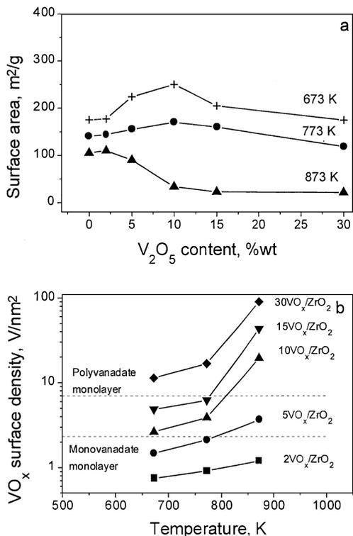
FIG. 1. Surface areas (a) and apparent VO<sub>x</sub> surface densities (b) of VO<sub>x</sub>/ZrO<sub>2</sub> catalysts calcined at different temperatures.
