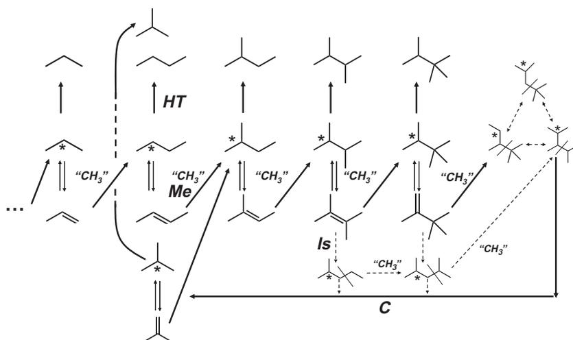
**Scheme 2.** Chain growth sequence for dimethyl ether homologation (starting with propene for simplicity). The asterisk indicates the position of alkoxide attachment to the surface. HT, Me, Is, and C labels represent hydrogen transfer, methylation, isomerization, and cracking reactions, respectively. “CH<sub>3</sub>” represents surface methylating species derived from dimethyl ether.
