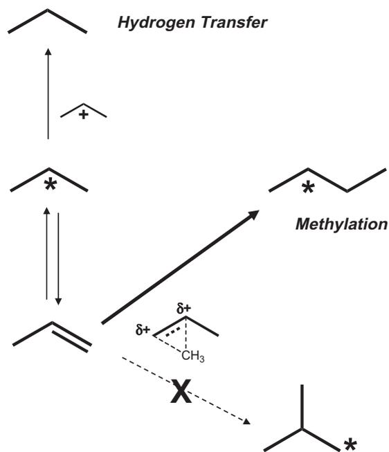
**Scheme 3.** Reaction pathways for C<sub>3</sub> species (propene and propoxide) in acid-catalyzed dimethyl ether homologation pathways. Methylation of propene occurs faster than hydrogen transfer to propoxide. Methylation of propene to isobutane does not occur because of the formation of a primary carbenium ion.
