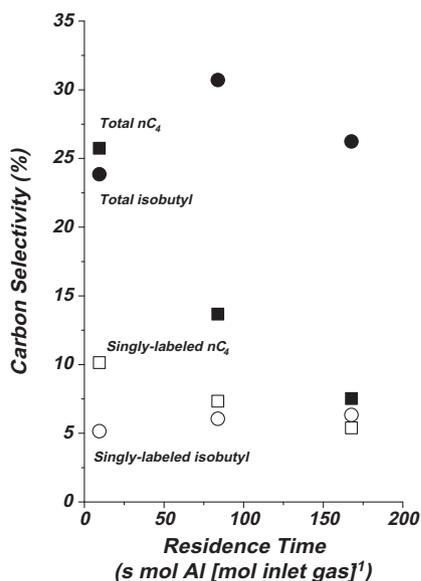
**Fig. 1.** Selectivity (% carbon basis) to linear C<sub>4</sub> species and isobutyl species as a function of reactor residence time (s mol Al [mol inlet gas]<sup>-1</sup>) for reactions between <sup>13</sup>C-labeled dimethyl ether (84 kPa) and unlabeled propene (2 kPa) at 473 K on H-BEA (Si/Al = 12.5). Total carbon conversions were less than 5%.
